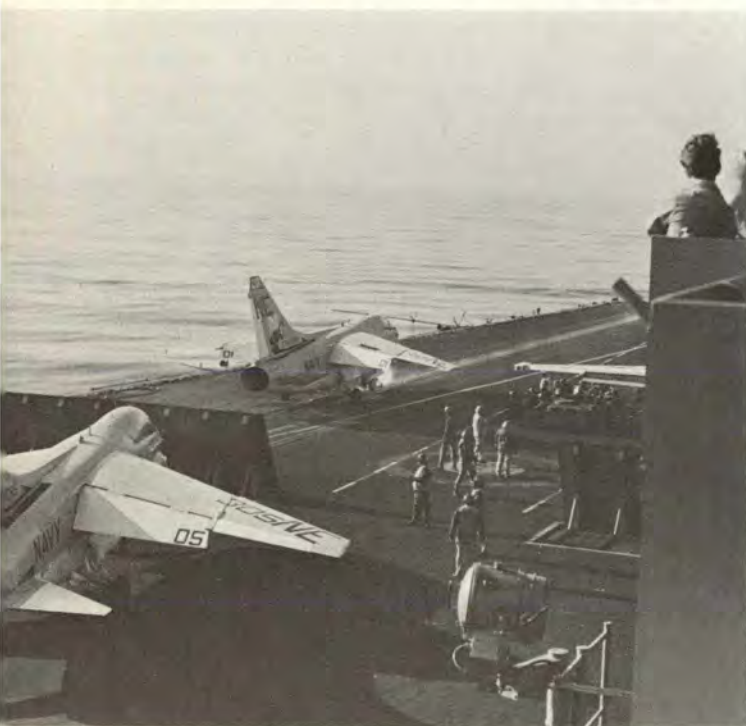
After each catapult takeoff, the tremendous amount of steam necessary to power the high speed tow escapes to the deck. The whole area goes IFR for several seconds as the crew readies that catapult for another launch.
