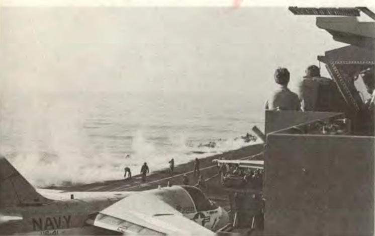
After each catapult takeoff, the tremendous amount of steam necessary to power the high speed tow escapes to the deck. The whole area goes IFR for several seconds as the crew readies that catapult for another launch.
